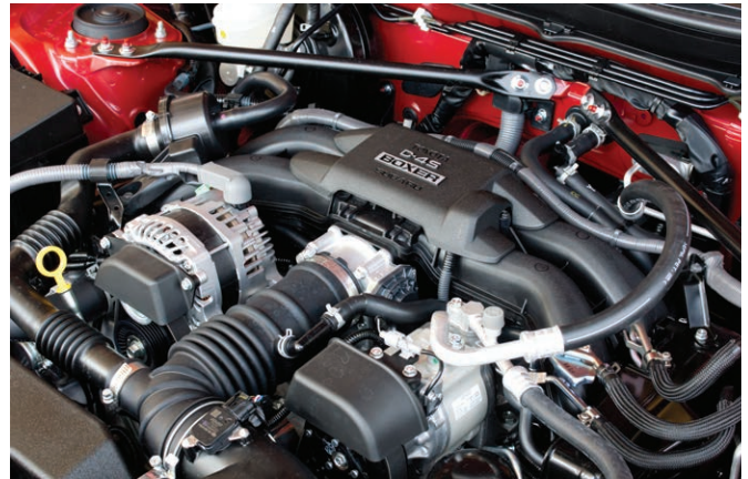
FIGURE 2-49 The Toyota D-4S system utilizes both a port fuel injector, along with a GDI high-pressure injector. When the vehicle is in cleaning mode, the PCM utilizes the port fuel injectors to clean the intake valve when engine operation dictates cleaning is required.
