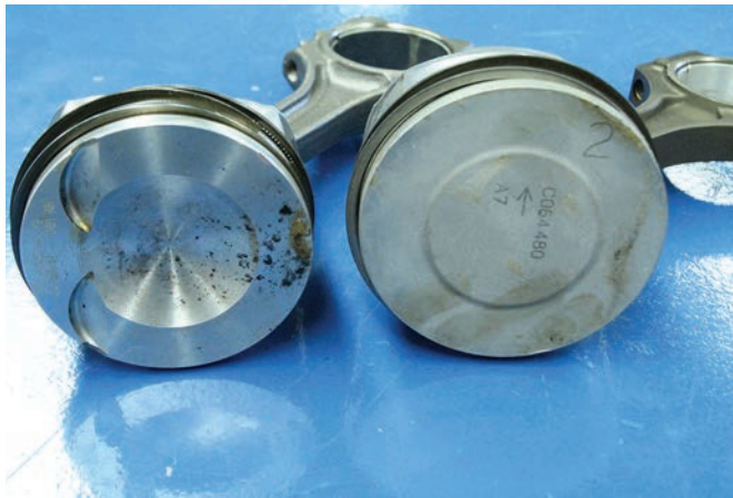
FIGURE 2-33 The design of a GDI piston helps disperse the fuel once it has been injected into the cylinder. When the fuel hits the piston, it atomizes to mix more with the air in the combustion chamber. This provides a more complete and powerful combustion event, which leads to more power and less emissions.
