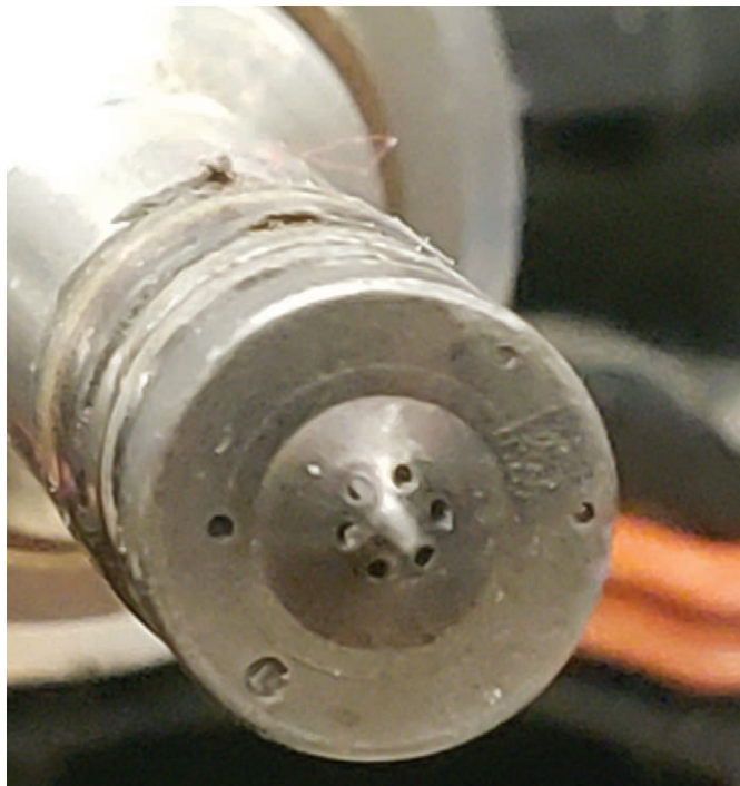
FIGURE 2-38 The machined holes in the tip of the injector help atomize and direct the fuel flow toward the correct location on the piston head. The pressure and direction allow for the piston head to control the splash and direct it toward the spark plug for a more complete combustion event.
