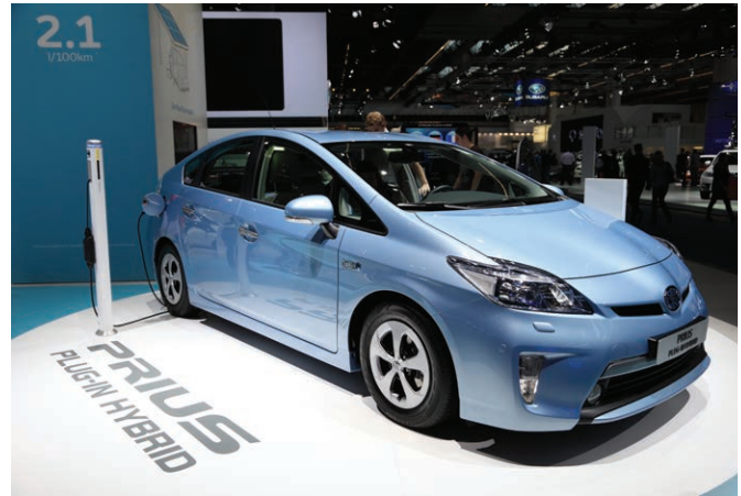
FIGURE 2-5 The plug-in hybrid electric vehicle (PHEV) is a combination of an HEV and a battery electric vehicle (BEV). It has the plug-in features of a BEV and the extended range of an HEV. The PHEV is a necessary evolution from an ICE-equipped vehicle to a vehicle fully powered by electricity.
