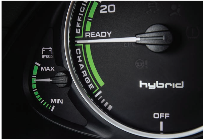
FIGURE 2-4 The regenerative braking system utilizes components that are already in the high-voltage system to generate electricity based on the vehicle in motion. The power used to make the stationary vehicle move to a particular speed can partially be recovered when the vehicle is decelerating. Energy does not disappear, it simply changes forms. Recapturing energy before or as it changes forms is an easy way to minimize the need for the battery pack to be charged externally.
