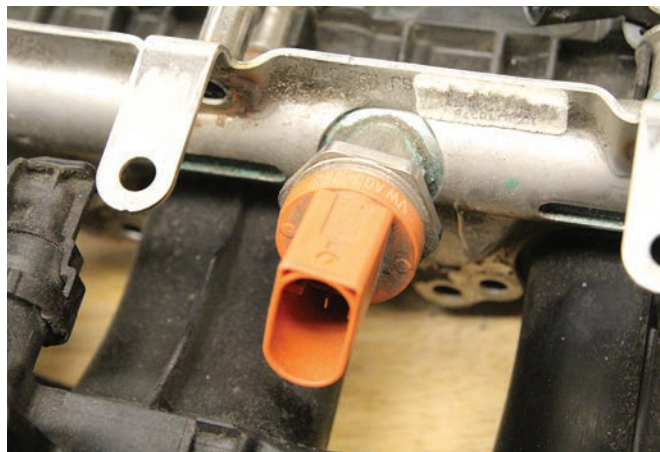
FIGURE 2-41 The high-pressure fuel sensor is used to monitor the fuel pressure on the high side of the fuel-injection system. This pressure is used by the PCM to change output of the pump to match the needs of the engine.
