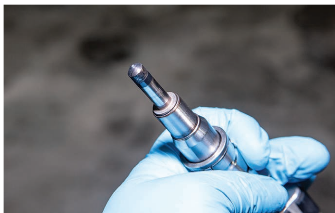
FIGURE 2-46 The buildup of carbon on the tip of an injector can cause the spray pattern to not match what is needed to promote proper combustion.
