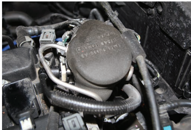
FIGURE 2-45 The noise-absorbing material is used to stop the fuel system noises from escaping the engine compartment.
