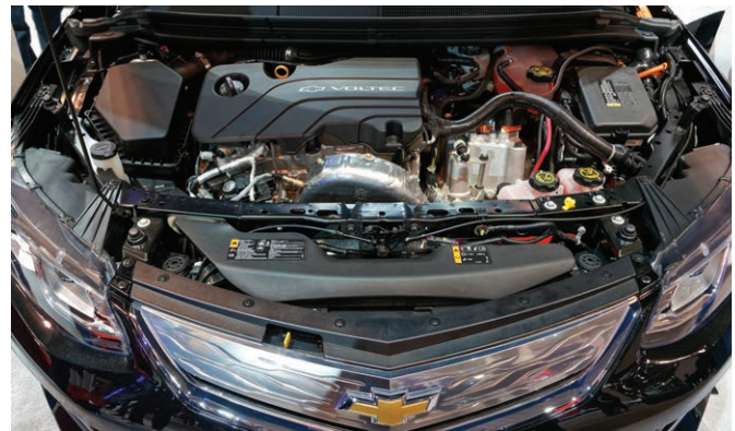
FIGURE 2-6 The propulsion system on a PHEV is much more complicated than that on a BEV. Integrating the ICE allows for extended range, but also increases costs for the owner of the vehicle. In a traditional ICE-powered vehicle, the owner only has to worry about the drivetrain of the vehicle for propulsion. In a PHEV, the owner has to worry about the drivetrain, high-voltage electronics, and the battery pack. The increased complexity dramatically increases the cost to repair.
