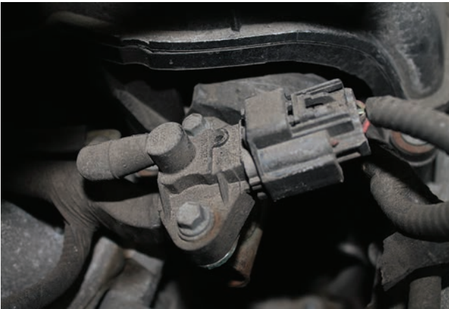
FIGURE 2-42 The high-pressure fuel sensor is a very simple transducer that gives feedback to the PCM so that it understands the amount of pressure that is present in the high-pressure side of the fuel system.
