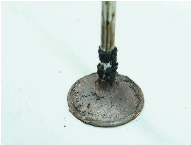
FIGURE 2-47 Carbon can keep valves from sealing correctly and cause a drivability issue. To fix this issue, the cylinder head may need to be removed in order to remove the valve and clean it.
