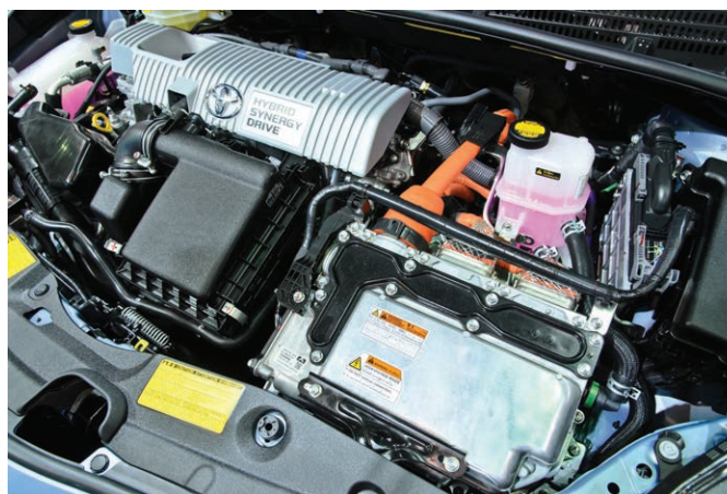
FIGURE 2-17 Some hybrid models use the Atkinson cycle because they are a stationary engine that does not have the violent rpm swings found in a conventional engine. The increased efficiency of this four-stroke strategy allows for increased fuel efficiencies that are not found in an Otto four-stroke engine.
