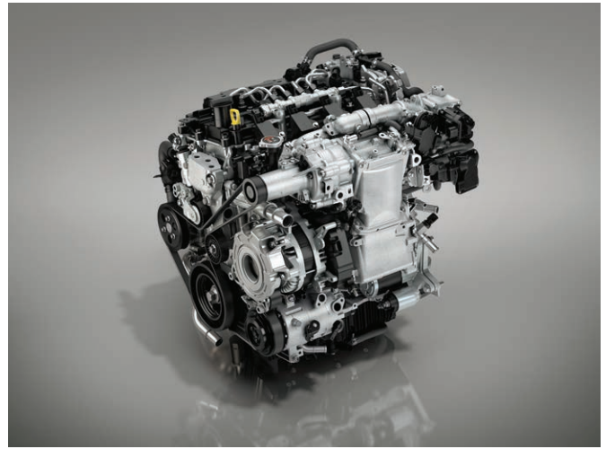
FIGURE 2-52 Mazda uses a hybrid type of homogeneous charge compression ignition (HCCI) engine that uses SI and CI types of technologies to increase the fuel efficiency and power of the engine. Used with permission from Mazda Motors Corp.
