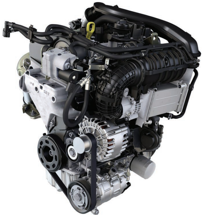
FIGURE 2-18 The Miller-cycle engine is based on the Atkinson-style engine but employs a supercharger and a delayed intake valve closing feature. These two features allow it to increase efficiency by up to 15%. Used with permission from Volkswagen AG.
