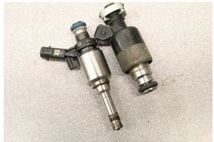
FIGURE 2-36 The port fuel injector is smaller than the GDI injector because it only has to reach the intake port to fill up the back side of the valve with fuel. The GDI injector has to reach all the way into the combustion chamber.
